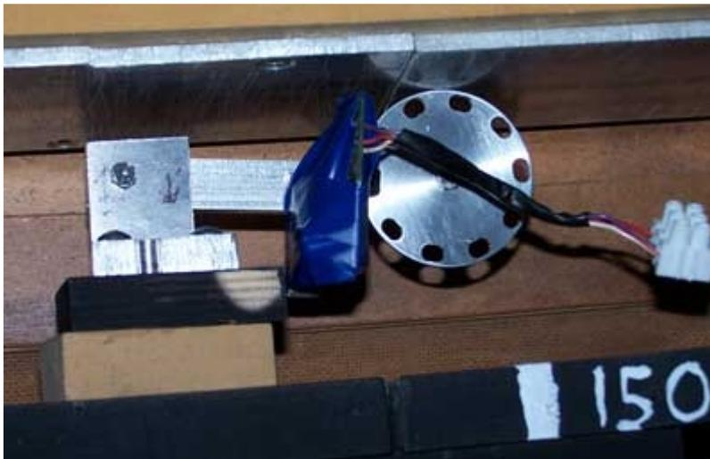
A 2 hole solution, notice that opto-sensor spacing is 45 degrees
