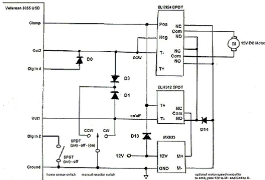
(1) ELK924 needs to be triggered in "insensitive" mode, (2) reverse-current protection diode D0 prevents the D14 circuit from triggering ELK924 all the time. If Out2 is pulled to 0V, current can flow from In4 to Out2 and be detected by the 8055 as an input signal. However, if Out2 is not enable, the diode prevents current from exiting the 12V circuit of ELK input, into In4, through the pullup resistor, to the 5V level. (3) motor speed control board MX033 allows rotation speed to be lowered.
