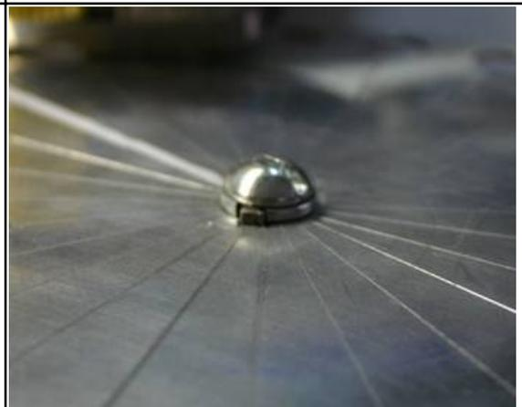
The commutator's drive shaft has a keyway 0.125 X 0.125 which is inserted into the commutator and acorn gear preventing unwanted independent rotation.
